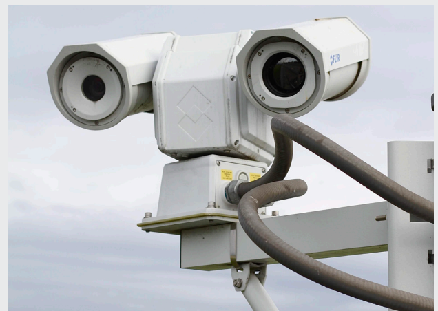
Combining a 640 x 480 resolution thermal sensor, a HD visible-light imaging sensor, and a high-speed precision pan-tilt system, the FLIR Triton PT-Series HD camera delivers superior detection and tracking.
